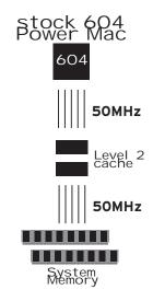
The magic of the PowerPC 750 chip is its ability to talk to the "backside" cache memory on the processor card at high speeds - up to the same speed as the clock of the CPU. The high number of cache "hits" makes the speed of the system bus almost irrelevant because the data is read from the cache memory at speeds far faster than the slower system bus.
